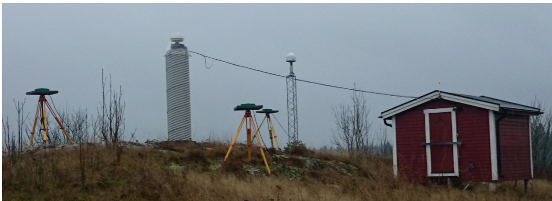
Fig. 1. The SWEPOS site Vänersborg during a station calibration setup in November 2014. An Eccosorb® plate is mounted directly below the visiting choke-ring antennas. Note the typical SWEPOS concrete pillar and the recent steel-grid mast with the LEIAR25.R3 antenna and LEIT radome installed.
