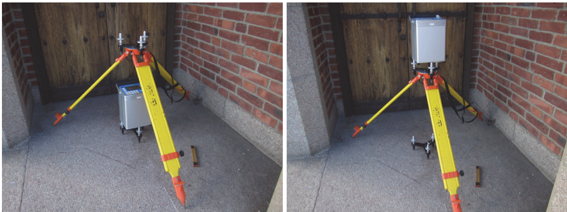
Fig. 8. Measurements for vertical gravity gradient determination at the Class B point Östersund AB, Sweden.
