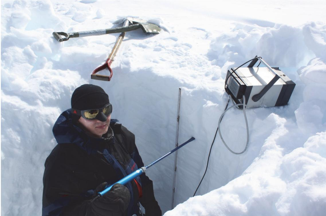
Fig. 4. Profiling the complex dielectric permittivity using the snow fork in a snow pit. The measurements provide estimates for the density and liquid water content of snow (*Sihvola and Tiuri, 1986*).
