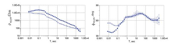
Fig. 5. Apparent resistivities and impedance phases from one day recording of the EMMA II array measurements in summer 2007 in Kuusamo-Pudasjärvi region in Finland. Dots represent xy component (geomagnetic NS), crosses yx (EW) component. Vertical bars show 95% confidence limits.
