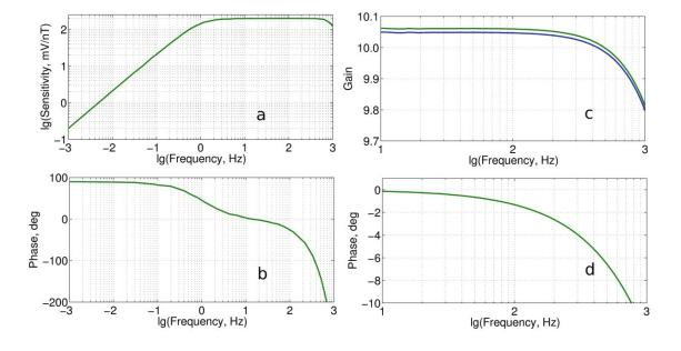
Fig. 4. Transfer functions of the two magnetic (H) channels (= difference between input and output signal as a function of frequency) and electric (E) channels. (a) Sensitivity of H channels, (b) phase of the transfer functions of H channels, (c) gain factor of E channels and (d) phase of the transfer functions of E channels.
