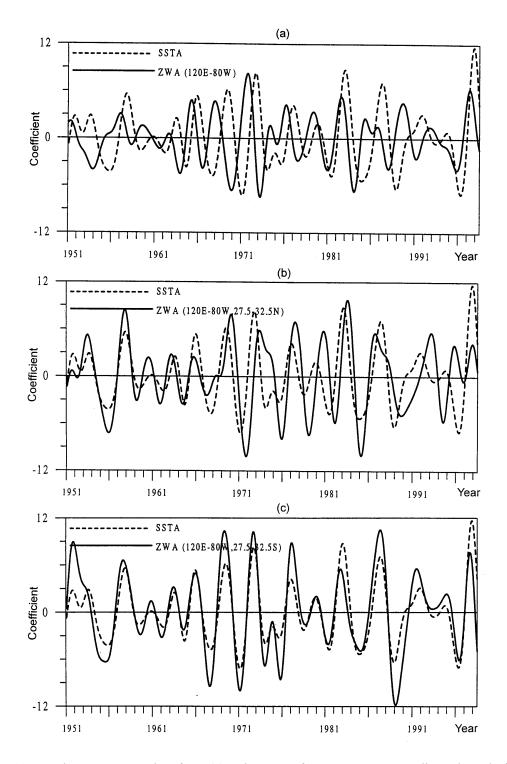
Fig. 11. Wavelet component series of NINO3 region sea surface temperature anomalies and zonal wind anomalies for regions of (a) the equatorial Pacific, (b) the north subtropical Pacific, and (c) the south subtropical Pacific at the 70-month time-scale.
