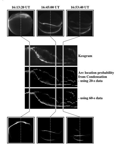
Fig. 8. Results from the tracker: individual images (top row), a time vs. latitude plot generated from the images (middle), and the arc location probability density from CONDENSATION projected onto latitude (bottom). Lighter colour indicates brighter aurora or more probable arc location. Images are from Kilpisjärvi, 1999/10/22 16:07–17:11 UT.
