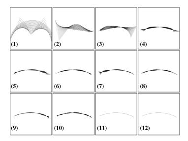
Fig. 7. Reducing shape variability by using PCA. The eigenmodes of the 12-dimensional arc shape sorted in decreasing order of eigenvalues: the first two eigenvectors capture approximate 92% of the variance in the data set.
