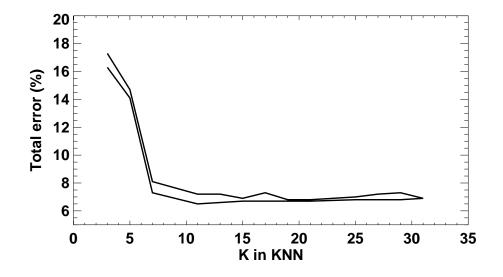
Fig. 5. The classification error as a function of K in KNN classification – upper and lower bounds are shown. The bounds are estimated by classifying all images (lower bound) and using a "leave-one-out"-technique (upper bound) (*Therrien*, 1989).
