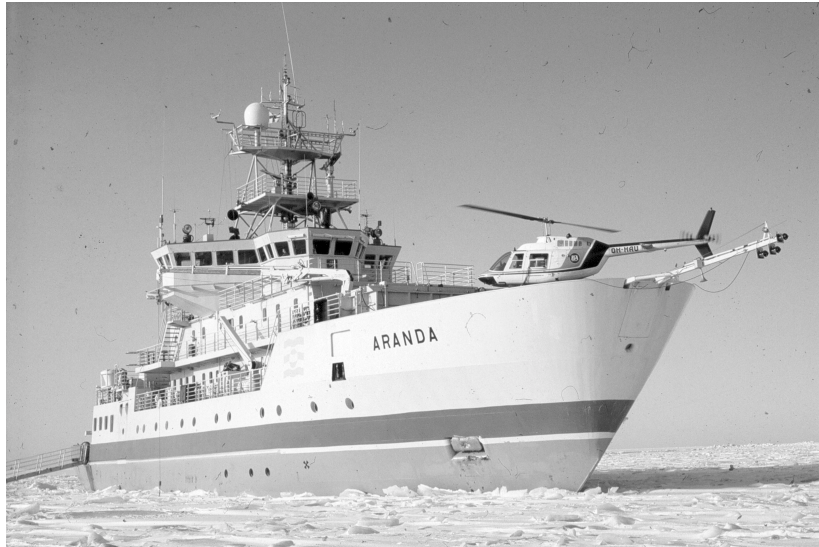
Fig. 6. R/V Aranda (III) at work in pack ice field. Helicopter landing on the front deck, light mast folded down.
