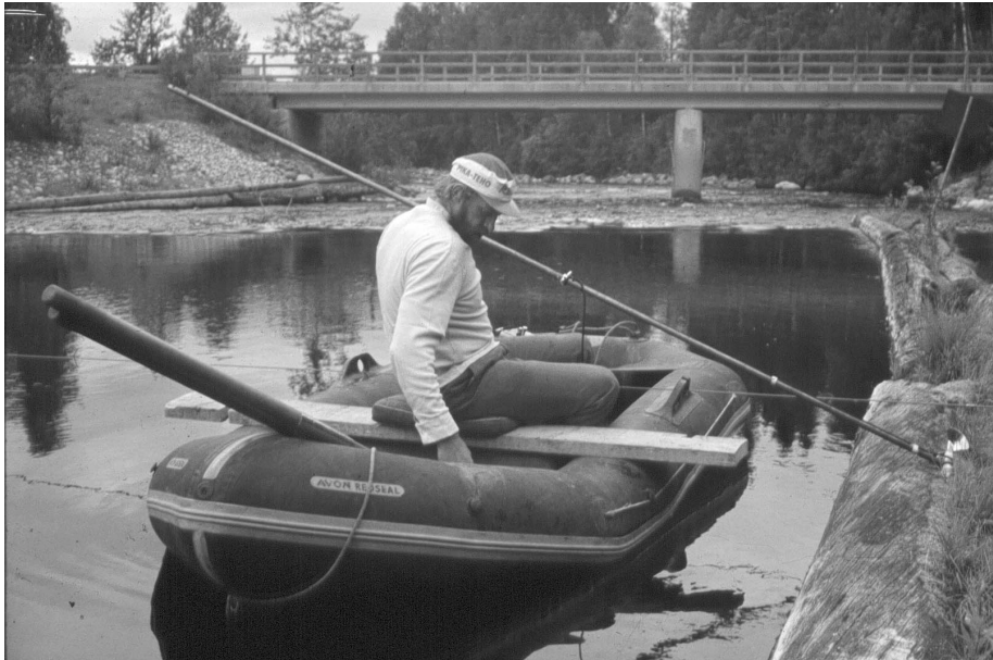
Fig. 5. A discharge measurement in Saramojoki River in Northern Karelia in the 1970s (photo by Esko Kuusisto).
