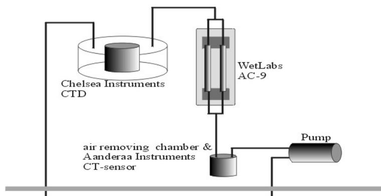
Fig. 1. Measurement setup in the r/v Saduria.
