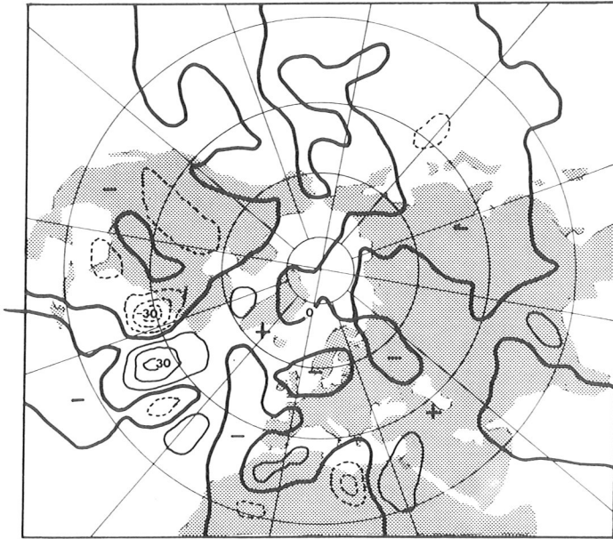
Fig. 9. Distribution of -\nabla \cdot H_2 (= -\nabla \cdot \frac{1}{2} (\overline{V' \cdot V'}) \bar{V}) averaged vertically. Unit: 10^{-4} \text{Wkg}^{-1} .
