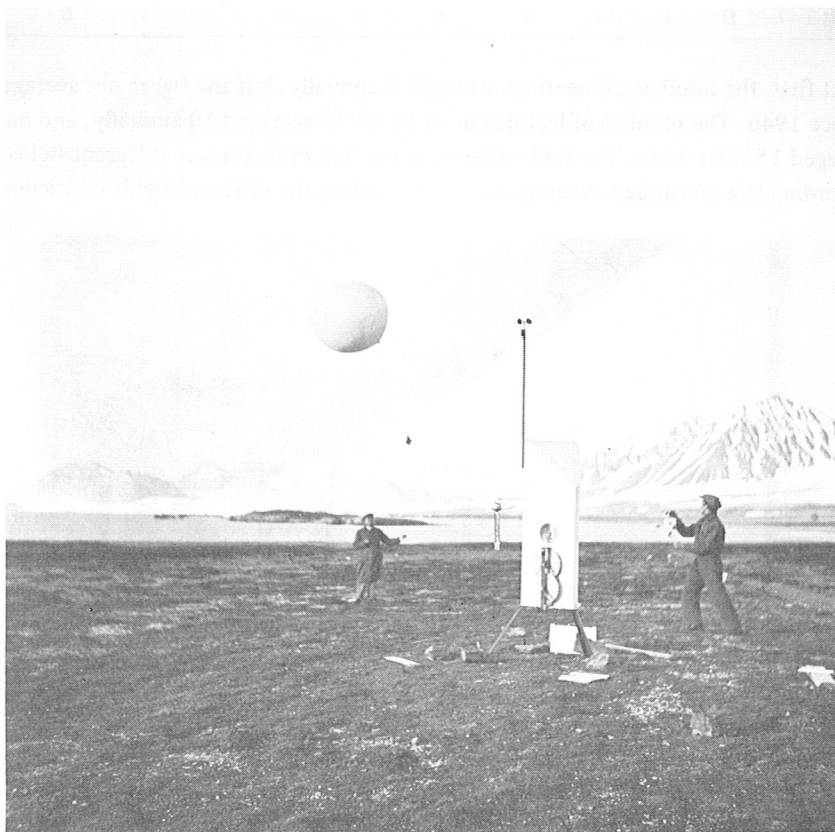
Fig. 5. Rawinsonde launch during the expedition to Spitzbergen in 1937.
