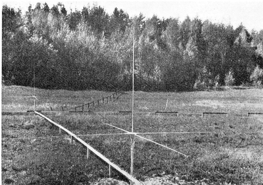
Fig. 2. Radiotheodolite antennas at the Testing Station of the Radiosonde Factory Vaisala Oy near Helsinki.
