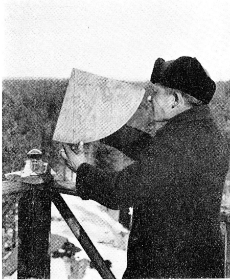
Fig. 15. Plumb quadrant in use for the determination of height angles, and a total pyranometer.
