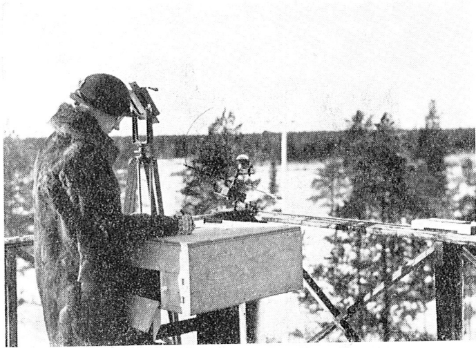
Fig. 16. Auroral camera, an illuminated box with a star map for visual auroral observations, the diffuse pyranometer and the grey-wedge photometer in the auroral tower.
